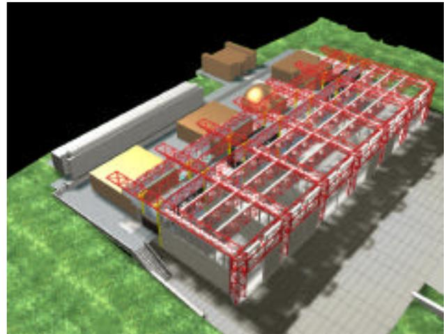
*Figure 4. Isometric of proposed facility showing structural elements*
