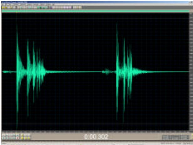
Figure 3. Two Typical Impact Waveforms as Displayed on Cool Edit 2000
