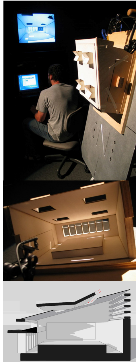
Figure 8a: Adjustable-table heliodon assessment; 8b: Video documentation of solar access; 8c: Proposed changes (shown red) for light shelf & top.
