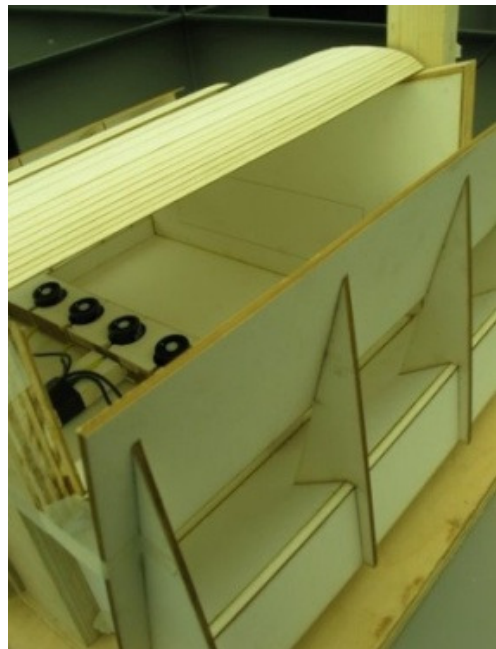
Figure 11: Illuminance measurements using five-sensor paddle.
