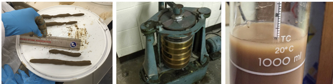
Figure 2: Soil sample analysis: cigar test (left), sieve test (center), and hydrometer test (right). Source: (Author)
