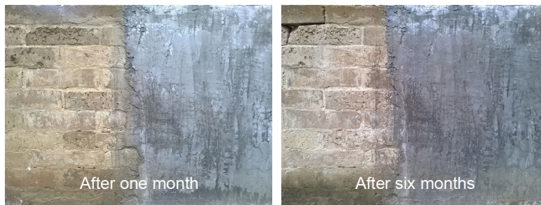
Figure 5: Earth block wall weathering, one month (left) & six month (right) durations. Source: (Author)
