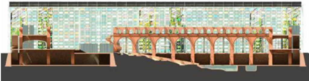
Figure 6: Palm House Natatorium in sections shows the utilization colored glass and exterior climbing plants as shading mechanisms that respond to changes in season and time of day. Opportunities for users to choose places to linger with nearly full, sun, filtered light, or full shade are present. Source: (Habtour)
