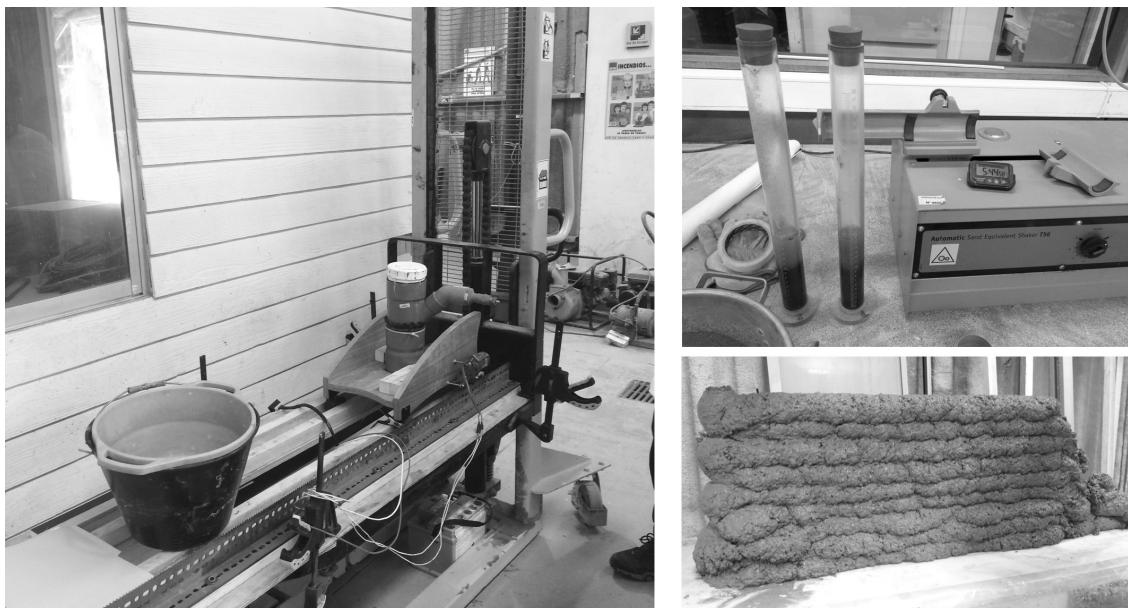
Figure 2: Left: equipment to test material deposition; Upper-right: evaluation of sands; Lower-right: sample of material deposition. Source: (Author 2018)
