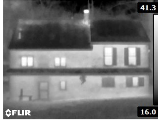
Figure 5. Full 160x120 pixel image, North wall at 6:59 AM
