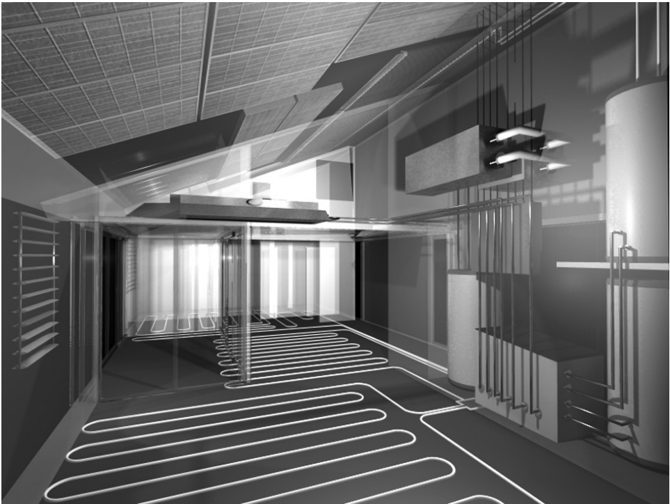
Figure 8: Visualization of heating and cooling system embedded into the building fabric. (Andrew Becker 2009)
