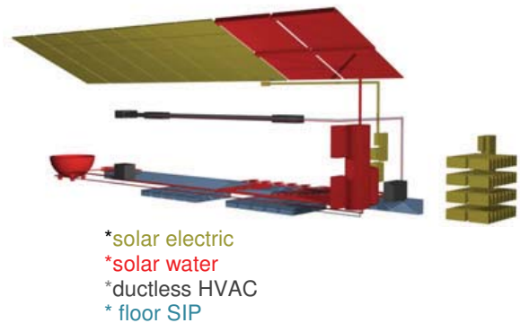
Figure 5: BLOOMhouse Mechanical Systems
