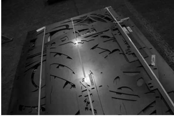
PANELS 1-F & 1-G WILL BE WELDED TO PANEL 1-D PATTERN ON PANEL 1-D INCLUDES SQUARE HOLE WITHIN THE PATTERN FOR ACCESS TO WELD PANELS & BOLT BRACKETS FROM CHIMNEY TO ROOF PANELS
